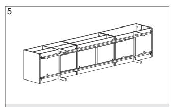
Use the screws (E) to connect the frame to the coupled bodies. Rotate the cupboard back on its frame.
