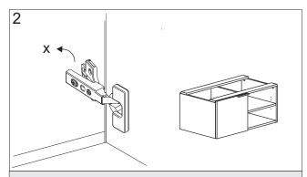
Remove the doors, if present. Remove the hinge from the panel. Do this by pulling lip x at the rear of the hinge forward. First, remove the damper.
