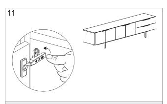
Replace the doors. Click the hinge back into the panel in the cupboard.
