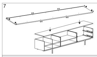
Place the minifix-pins C (see \*) and dowels D (see  $\bullet$ ) into the finishing top. Place the finishing top on the bodies and fix them by a half turn of the minifix-bush.
