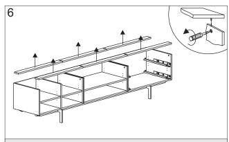
Dismount the transport laths by a half turn of the minifix-bush. Screw the minifix-pins out of the transport laths.
