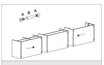
Rotate the bodies 90 degrees with the back to the ground. Couple the bodies with bolt A and bush B.
