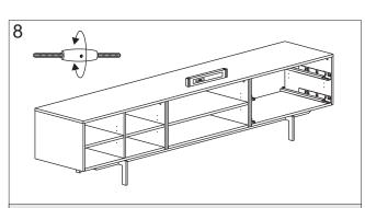
Place the cabinet in the desired position and level it by turning the adjustable feet by using the conical pin. To prevent the sideboard sagging under excessive loads, tighten the turnbuckles under the sideboard.
