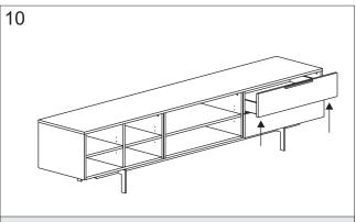
If necessary, the height of the drawer can be adjusted by means of the wedges underneath the drawer.
