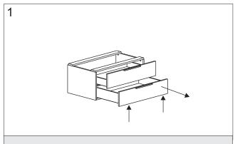
Remove the drawers, if present. To do this, grip the snappers on the underside of the drawer and pull it forward.
